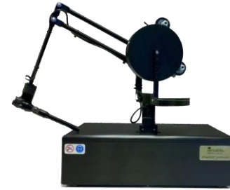
Figure 2: Control devices that fly the end effector can result in the robot moving to unintended orientations
